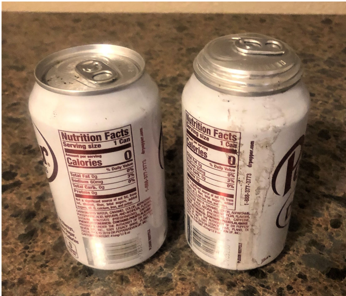
Two soda cans. The soda can on the right was left in the freezer.
